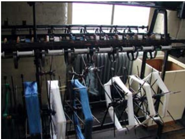
Next to this, a creel with bobbins of yarn ready to be wound onto a warping drum with heck block:
