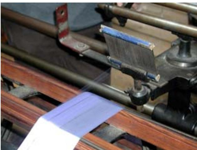
A view of the rows and rows of foot-powered jacquard looms. The first machine in the right-hand row is a tying machine – it was used to tie a new warp onto an old one. Before this was developed, it took a child worker (they've got the smallest hands) three days to tie on the new warp; with the machine, the task could be accomplished in half a day.
